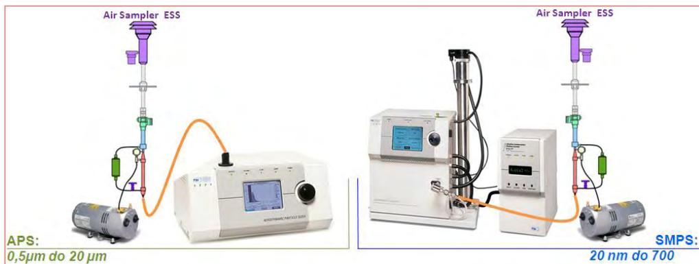
Fig.1. From left: The APS spectrometer with conditioning system; Spectrometer SMPS with conditioning system
