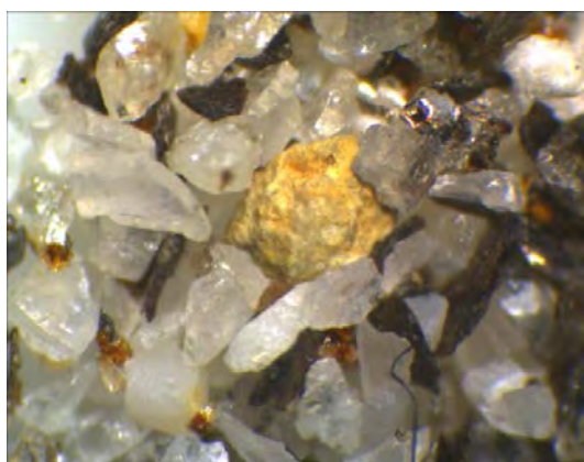
Figure 1. Concentrate of gold gets with flotation
