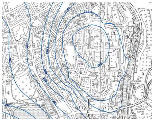
Figure 3. Cone of depression, groundwater level of 2004 (changed after LfULG 2005)
