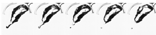
Figure 4. Sequence of images (2 ms apart) showing bubble formation in MIBC 7 ppm
