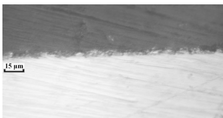
Figure 3. Metallographic cross section of Nimonic 901
