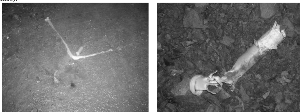
Figure 1. Control charge remaining in its place and marks of matrix (left) and outburst of the pipe with unsensitized matrix after firing of detonator (right) [5]
