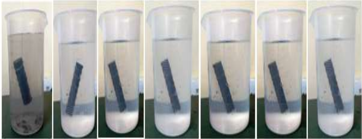
Fig 2. Fresh sample immersed in mine water, RO water and 1% to 5% NaCl solutions
