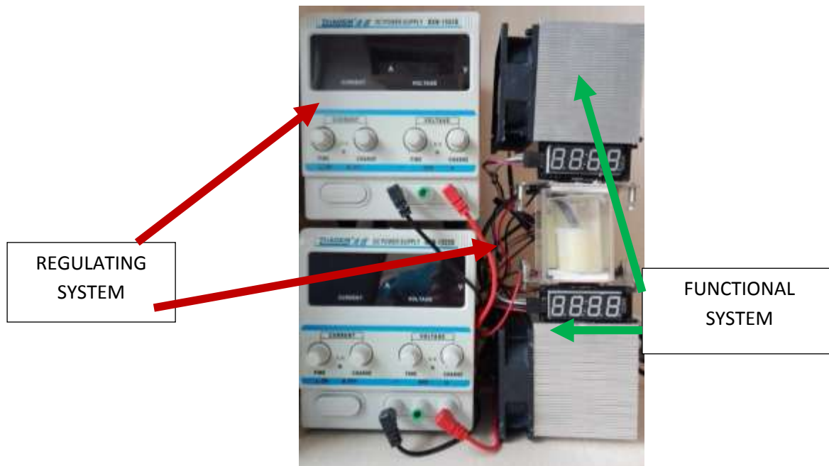
Fig.1. Photo of a testing station for phase-change material
