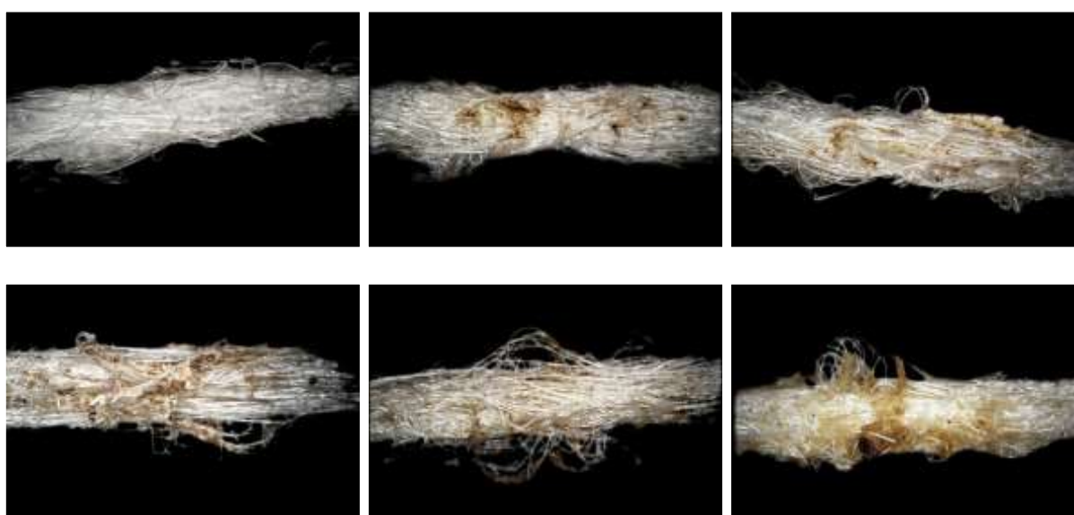
Figure 2: PESH + PA6-1 fiber after: 0, 18, 40, 90, 162 and 234 h cultivation with real waste water from a municipal sewage treatment plant.
