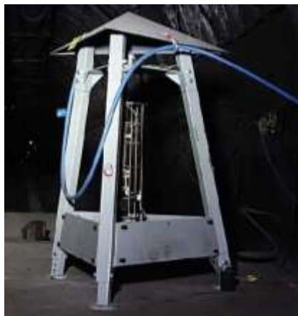
Figure 1 water measuring probe with frame in the mine “Auguste Victoria” (Germany, Marl)
