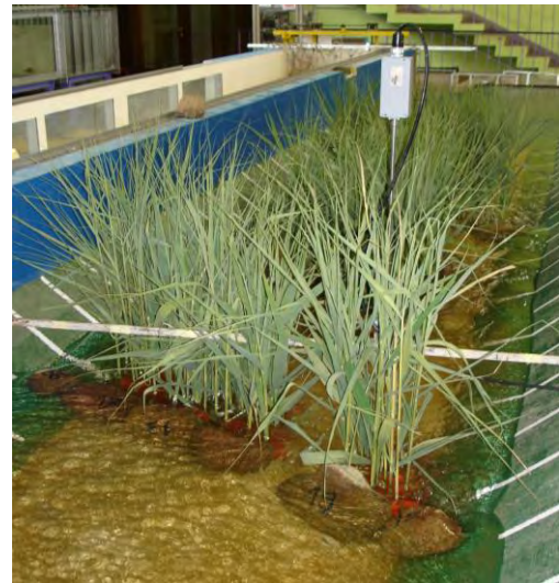
Figure 2. Measurements of local field of velocity by probe PEMS
