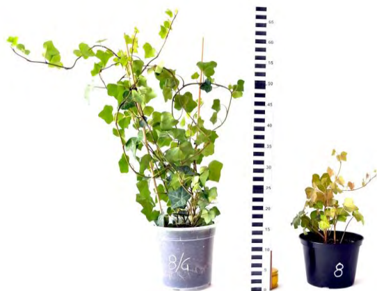
Figure 5. Plants planted at the same time with the same watering frequency. On the left side is plant with geocomposite. On the right side is the plant without geocomposite.
