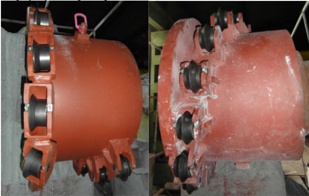
Fig. 2. Cutting head armed with asymmetrical disc (left) and symmetrical disco (right)
