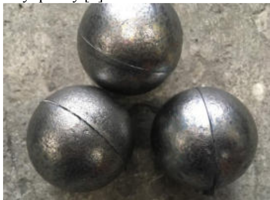
Figure 1 - Cast Iron Grinding Balls
