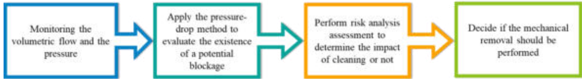
Figure 1 - Methodology to establish the predictive maintenance program
