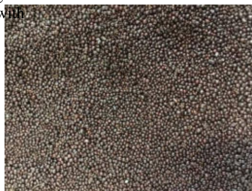
Figure 2 - Propants with diameter of 0.6 - 1.0
