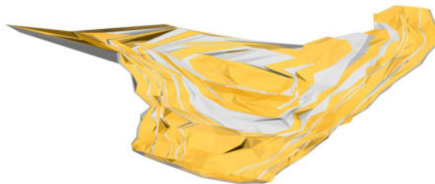
Figure 2 - Visualization of lithological differences of the Taldinskoye deposit site (all layers are colored in gray, and interlayers and combinations of mudstones, siltstones and sandstones – in orange)
