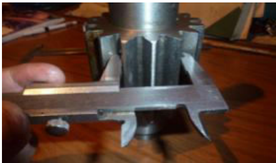
Figure 1: Checking the gear teeth "K" using a universal caliper
