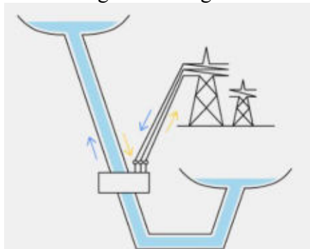
Figure 1 - The Principle of operation of HPSPP
