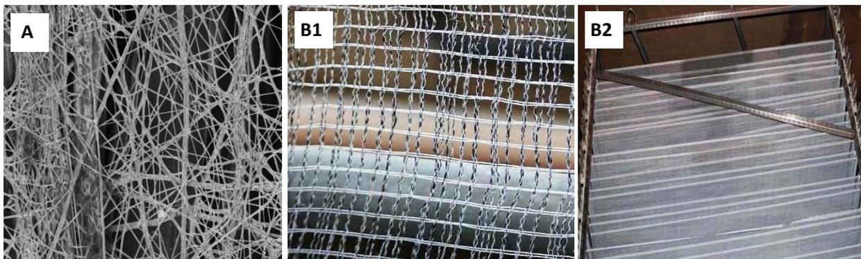
Figure 1. Nanofibers biomass carriers: A) picture of nanofiber from scanning electron microscope; B1) final textile; B2) supporting construction with textile.
