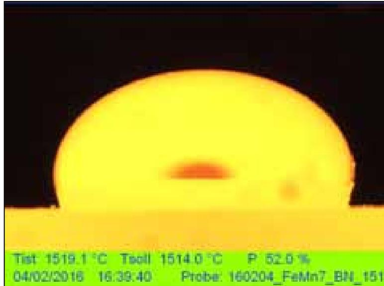
Figure 5. The image of a Fe-Mn binary (7 % Mn) on a BN substrate at 1519 °C temperature
