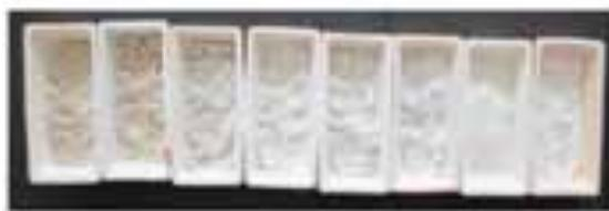
Figure 2. Residues of various density products (from  $<1.3$  to  $>2.0 \text{ g/cm}^3$ ) after being calcined
