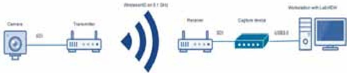
Figure 2. General scheme of machine vision system
