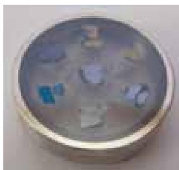
Figure 5. Polished reference block containing grains of Cu-sulfides (diameter: 2.5 cm)
