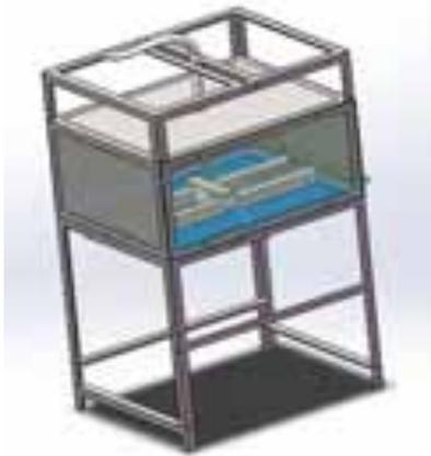
Figure 2. 3D Design of the gas environment cutting bench
