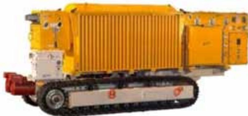
Figure 2. View of mobile power supply and maneuvering device EH d31 / d12-2100 / 6.0 / 1.0 / W / III / 02.21
