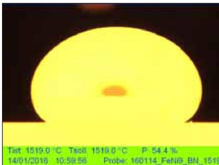
Figure 3. The image of a Fe-Ni binary (9 % Ni) on a BN substrate at 1519 °C temperature
