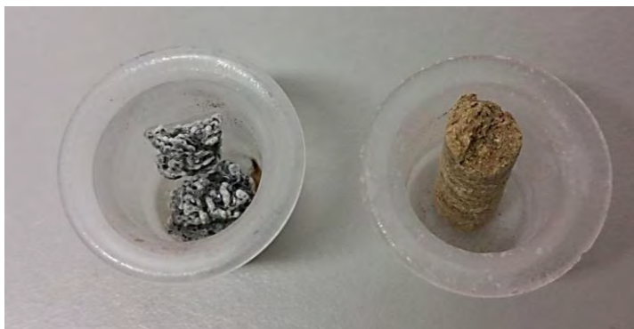
Figure 1. Experimental complete combustion product of 8mm rice husks pellets
