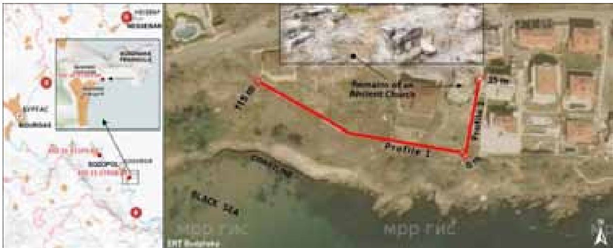
Fig. 2. ERT profiles of the landslide in the Budzhaka peninsula.
