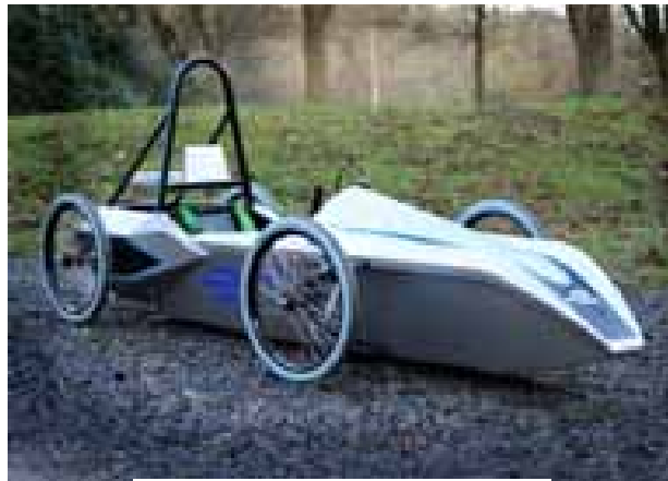
Fig 4. Greenpower class electric car
