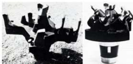
Figure 3: Multiple wing boring heads with flat chisels (left) and conical picks (right) [4]
