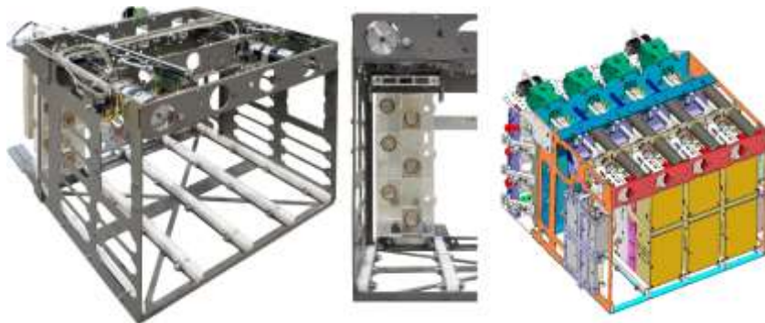
Figure 3. Construction frame for the insertion of contactor panels.
