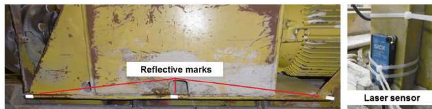
Figure 4: Measurement system to determine the drilling speed
