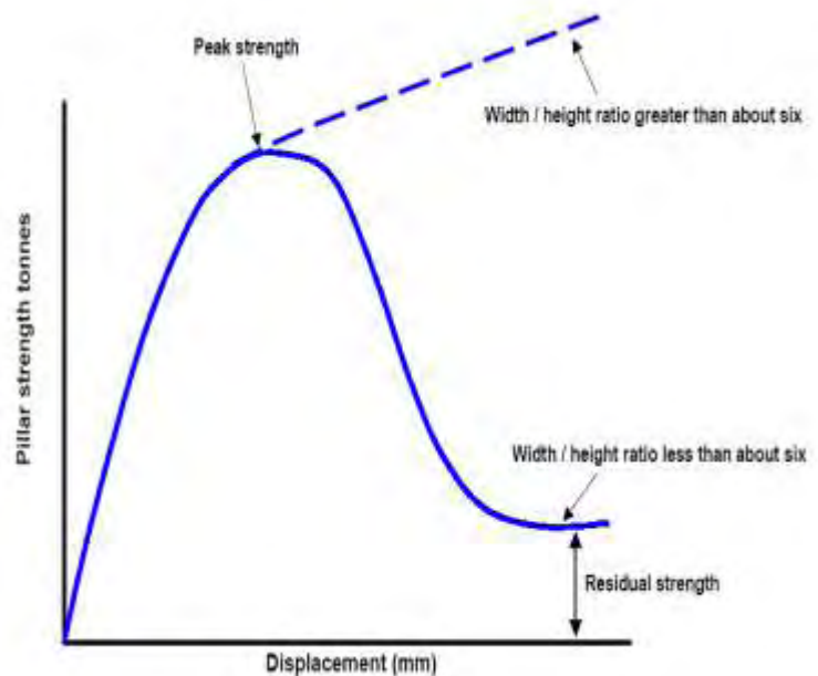
Figure 2. Typical Pillar Loading Behaviour Diagram (Hurt and MacAndrew, 2000)
