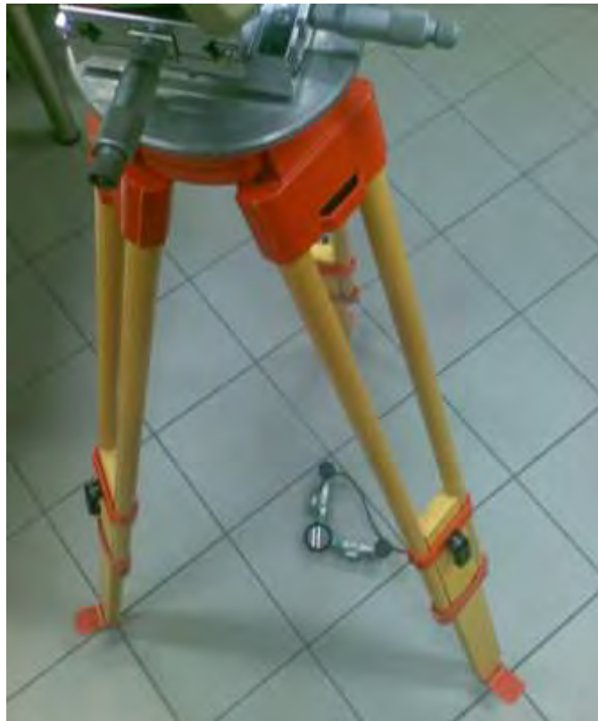
Figure 3. Electronic tachymeter TC1800 centering over reflective optical fiber adapter
