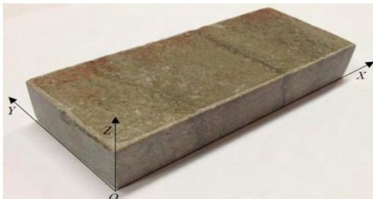
Fig. 1. Establishing of the coordinate system for acid rock sample
