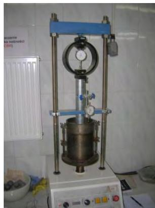
Photo 2. CBR rate testing machine
