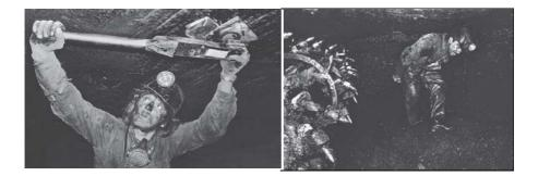
**Figure 1-2.** Coal miners face many occupational health and safety risks, including injuries and exposure to hazardous dusts, gases, and other substances. (A) Coal miner tests the roof support bolts in a mine. (B) Coal miner is exposed to ergonomic hazards from working in narrow mine passages.
