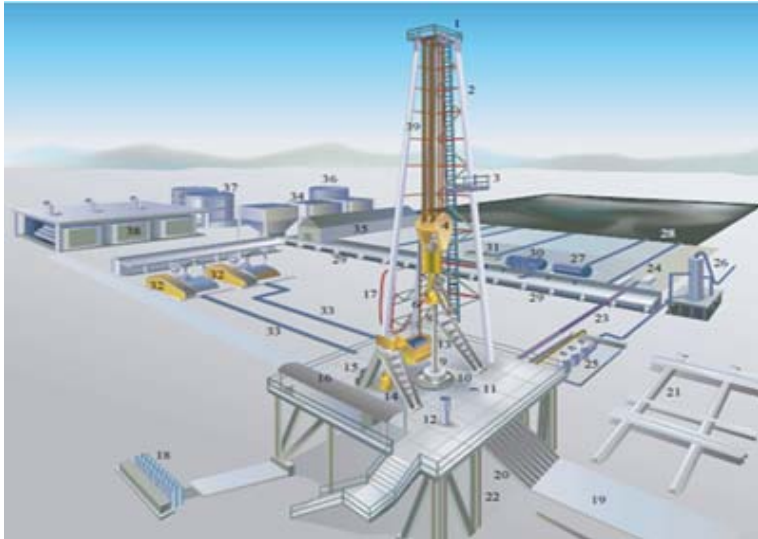
Fig.2 Main Equipment of a Rotary Drilling Rig
